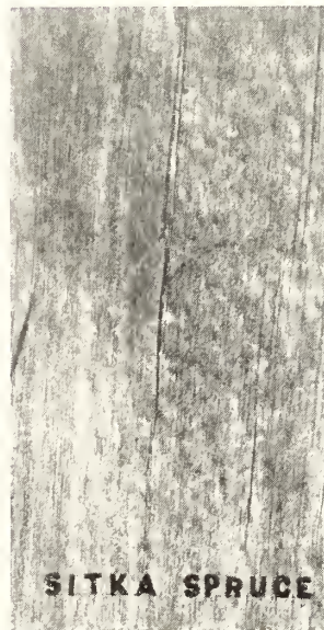
FIGURE 2-39.—Split tangential surfaces of Sitka spruce and Douglas-fir showing the "pocked" appearance of the spruce, not found in Douglas-fir. This characteristic is most pronounced in Sitka spruce with narrow rings and is almost entirely absent in very wide-ringed material.
